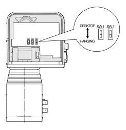
• If the pan/tilt head is connected to the multiport hub with a cable longer than 300 meters, set the cable compensation switch on the pan/tilt head to the ON position in advance. If the distance between the pan/tilt head and the control panel is shorter than 300 meters, keep the switch in the original position (OFF). For details on shifting the switch, refer to the figure below or the Operating Instructions for Pan/tilt Head.
