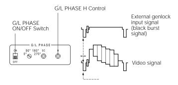
3 Set G/L PHASE ON/OFF Switch 6 back to the OFF position.
